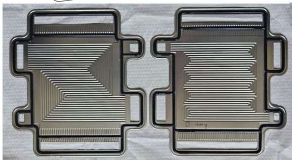
Anode and cathode plates with 50cm 2 active area
