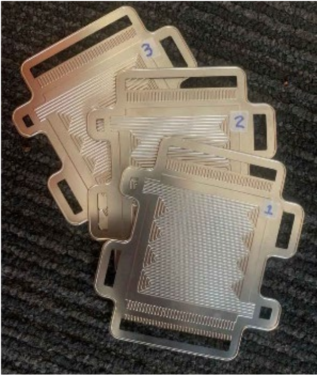
Final anode plates – 0.1mm thick titanium
