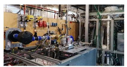
NOW GmbH supported solid oxide fuel cells are being tested for the production of onboard power for ships operating at sea and at berth in ports.
